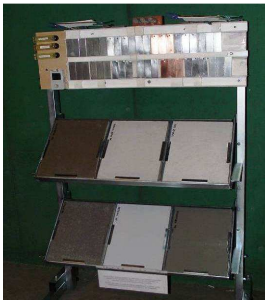
Rack with samples and sensors exposed at Mrazovka tunnel
