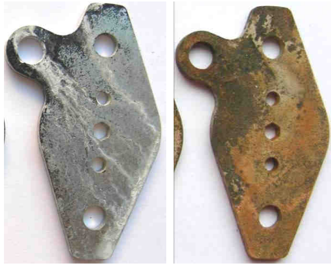
Figure 9: Component with Zn-Ni alloy coating corrosion attack after 600 hrs of NSS test (left) and 5 cycles in test with SO 2 (2 L dosage) (right)
