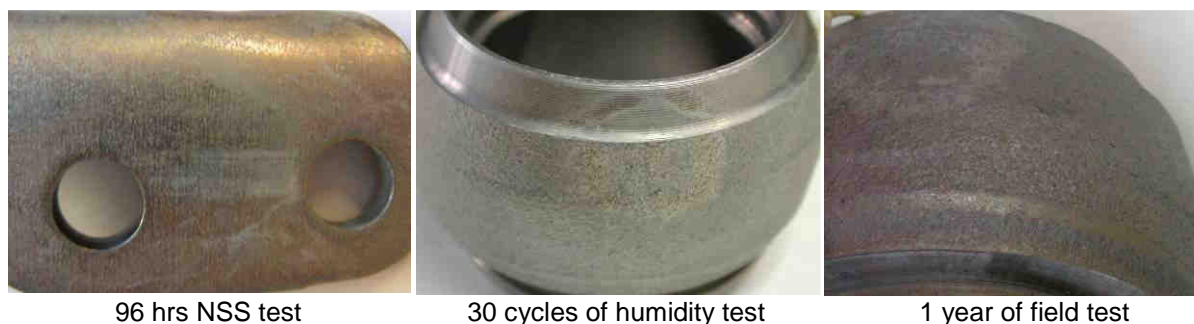
Figure 1: White-grey veil formed in different corrosion conditions
