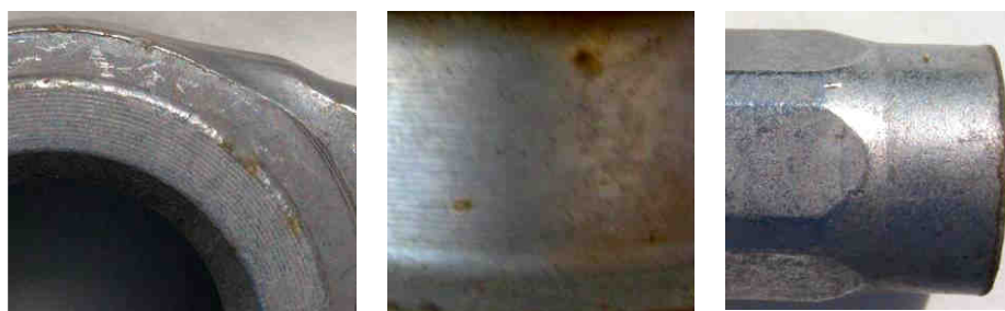
Figure 2: The corrosion of substrate steel after 3 months exposure on atmospheric test site
