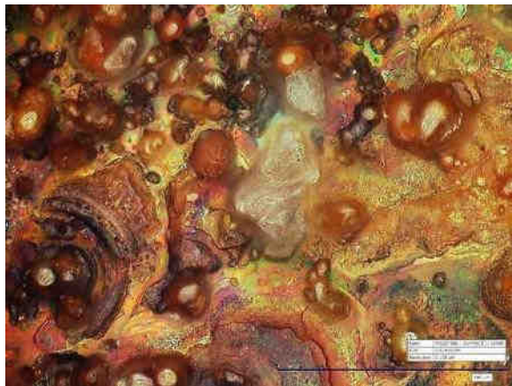
carbon steel, 2 months in tunnel
