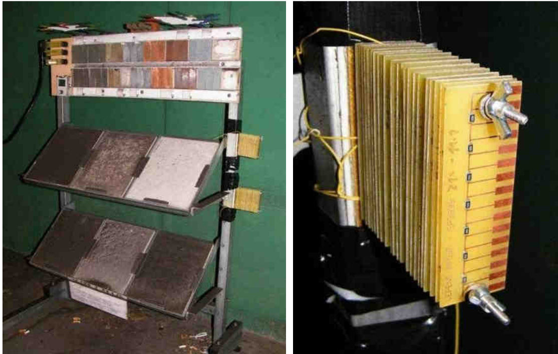
Figure 11: Rack with passive samplers and exposed metal coupons, resistive sensors and PCB with SMD attachments
