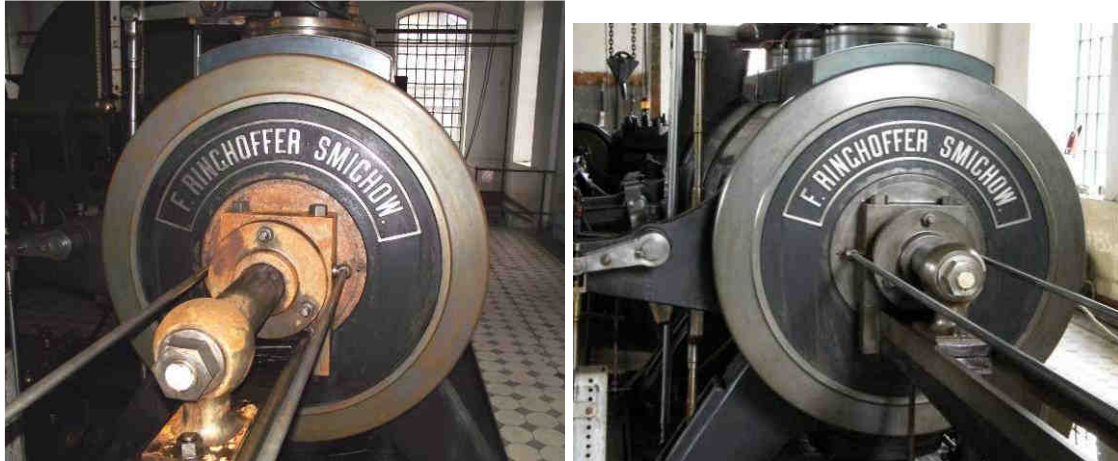
Figure 5: Example of steam engine before and after conservation (1 year left without regular maintenance)
